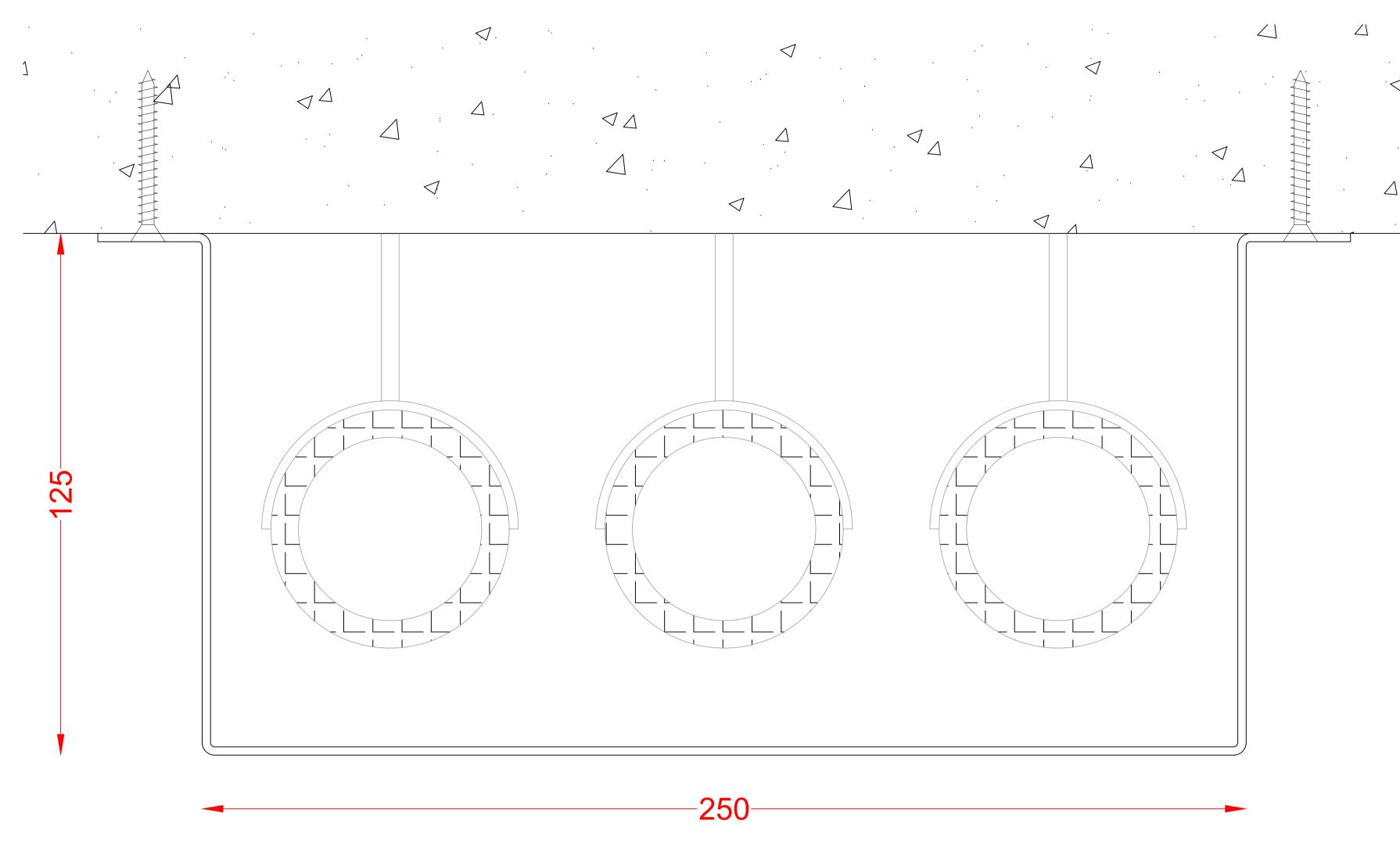
Services Void (Pipework, Cables etc)
