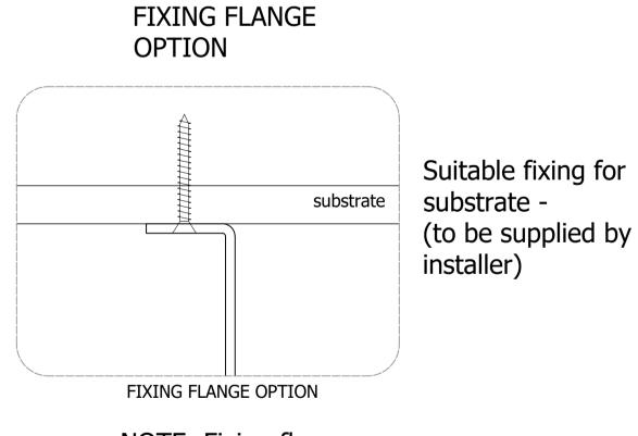
NOTE: Fixing flange option requires completely plumb / level substrate to avoid profile distortion
