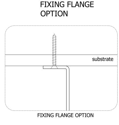
NOTE: Fixing flange option requires completely plumb / level substrate to avoid
